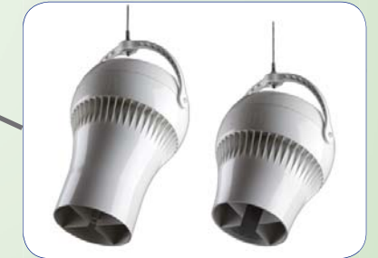
Air Pear fans return rising hot air back down through void in winter. Moderates air temperatures, provides particle ionisation to improve air quality and reduces air conditioning use.
